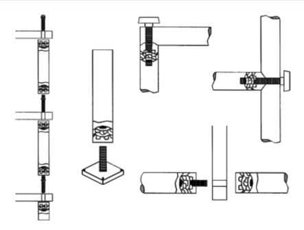
Inside Tube Diameter = 28,4-29,8Outer tube diameter = 1 1/4" Thread = M6
